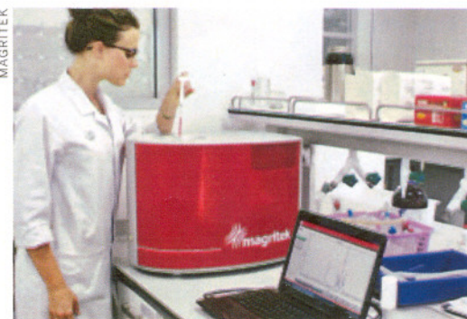
MAGRITEK The Spinsolve compact NMR spectrometer in a university chemistry laboratory.
